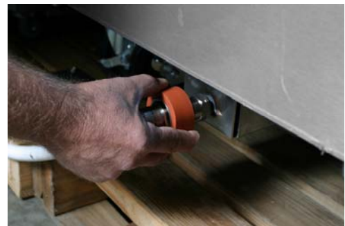
Optional hose/wand disconnect properly connected to disconnect valve in fryer cabinet.
